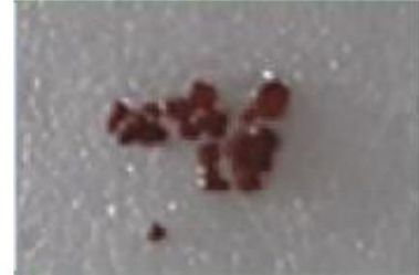
Residual fragments of a hard brick stone after shockwaves with the High Fragmentation Shock Head (only 738 shocks)
